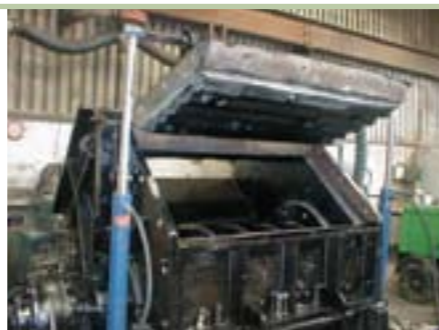
Manual prop should also be used in case of hydraulic lift-ram failure
